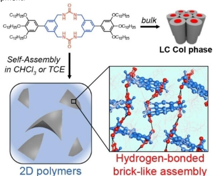
Figure 1. Dendronized bis-urea macrocycle forms columnar liquid-crystalline phases, while in solvents it self-assembles into two-dimensional (2D) nanosheets with a brick-like organization.
